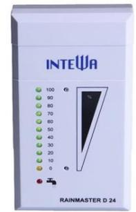
For rainwater systems using a submersible pump, the Rainmaster D24 can also automatically operate a solenoid valve, controlling the supply of mains water top-up to the tank, should the rainwater level in the tank run low. On activation, the mains water is passed through a so-called "air gap", as per DIN EN1717 regulations (European potable water safety regulations), and from there to the tank via a pipe.
