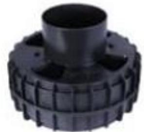
The incoming water falls straight down the inlet pipe and is turned 180 degrees upwards exiting out the small holes in the top of the calmer. In this way, even if the tank is empty, upward pressurised water cannot stir up sediment on the bottom of the tank. If not disturbed, the sediment compacts on the tank bottom and does not cause future fouling problems.
