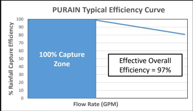
After this point, a hydraulic jump is created to vigorously clean the filter screen. Since most rain in any geography falls at a low flow rate, PURAIN has a big advantage at catching this water. All other self-cleaning filters lose some water at low flow rates. See specification sheet and website for more details.
