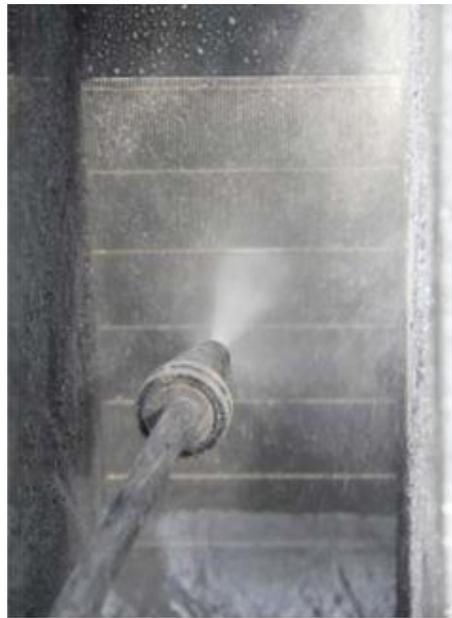
*Fig. 16: Automatic cleaning with high pressure cleaner*
